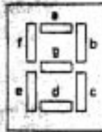
(a) Arrangement of Vertical and Horizontal Bars Needed to Produce the Decimal Digits Zero Through Nine. The Bars are Referred to as "Segments," and are Labelled 'a' Through 'g'.
