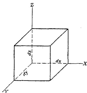
$$\nabla^2 \phi = \frac{\partial^2 \phi}{\partial x^2} + \frac{\partial^2 \phi}{\partial y^2} + \frac{\partial^2 \phi}{\partial z^2}$$
