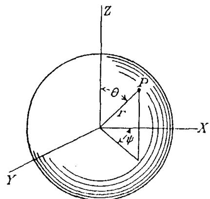
$$\nabla^2 \phi = \frac{1}{r^2} \frac{\partial}{\partial r} \left( r^2 \frac{\partial \phi}{\partial r} \right) + \frac{1}{r^2 \sin \theta} \frac{\partial}{\partial \theta} \left( \sin \theta \frac{\partial \phi}{\partial \theta} \right) + \frac{1}{r^2 \sin^2 \theta} \frac{\partial^2 \phi}{\partial \phi^2}$$
