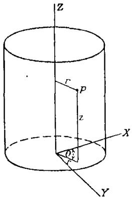
$$\nabla^2 \phi = \frac{1}{r} \frac{\partial}{\partial r} \left( r \frac{\partial \phi}{\partial r} \right) + \frac{1}{r^2} \frac{\partial^2 \phi}{\partial \theta^2} + \frac{\partial^2 \phi}{\partial z^2}$$
