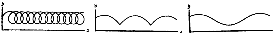
รูป 4.16 orbits in xy -plane of charged particle subject to a magnetic field in the z -direction and on electric field in the y -direction
