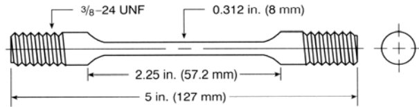
(b) Threaded-end tensile test specimen
